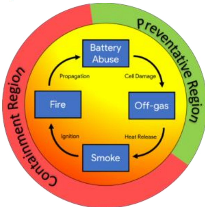
Figure 3-2 Thermal runaway cycle
